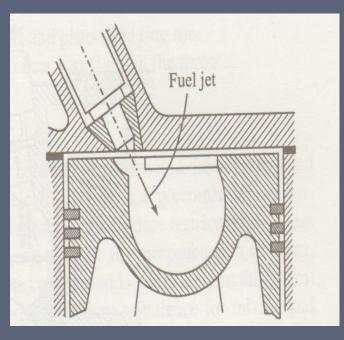
. In practice, this engine gives good performance even with fuels of exceedingly poor ignition quality. Its fuel economy appears to be extremely good for an engine of small size. Because of the vaporization and mixing processes, the 'M' engine is ideally suited as a multi-fuel engine.
