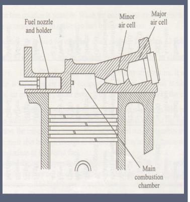
• In this type of the engine, the fuel consumption is higher and more energy is carried away in the exhaust and cooling water. Thus the life of the exhaust valve is reduced and this engine requires larger radiator and fan.
