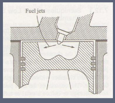
Figure shows a bowl-in-piston type of medium swirl open chamber with a centrally located multihole injector nozzle. The amount of liquid fuel which impinges on the piston cup walls is kept minimum. This type is used in medium size (10 to 15 cm bore) diesel engines.
